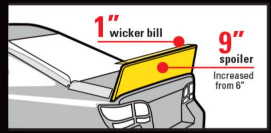
THE INCREASED DOWNFORCE ADDS DRAG TO THE CAR AND CREATES A LARGER DRAFT WINDOW IN THE BACK.
